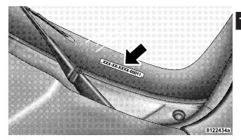
**Vehicle Identification Number NOTE:** It is illegal to remove the VIN.
